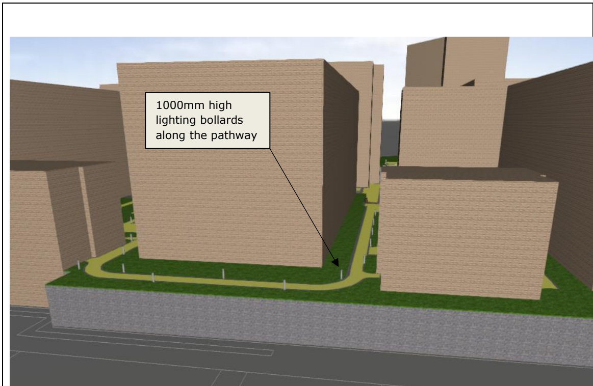
Fig 1 - 3D - Typical Location of Bollard
